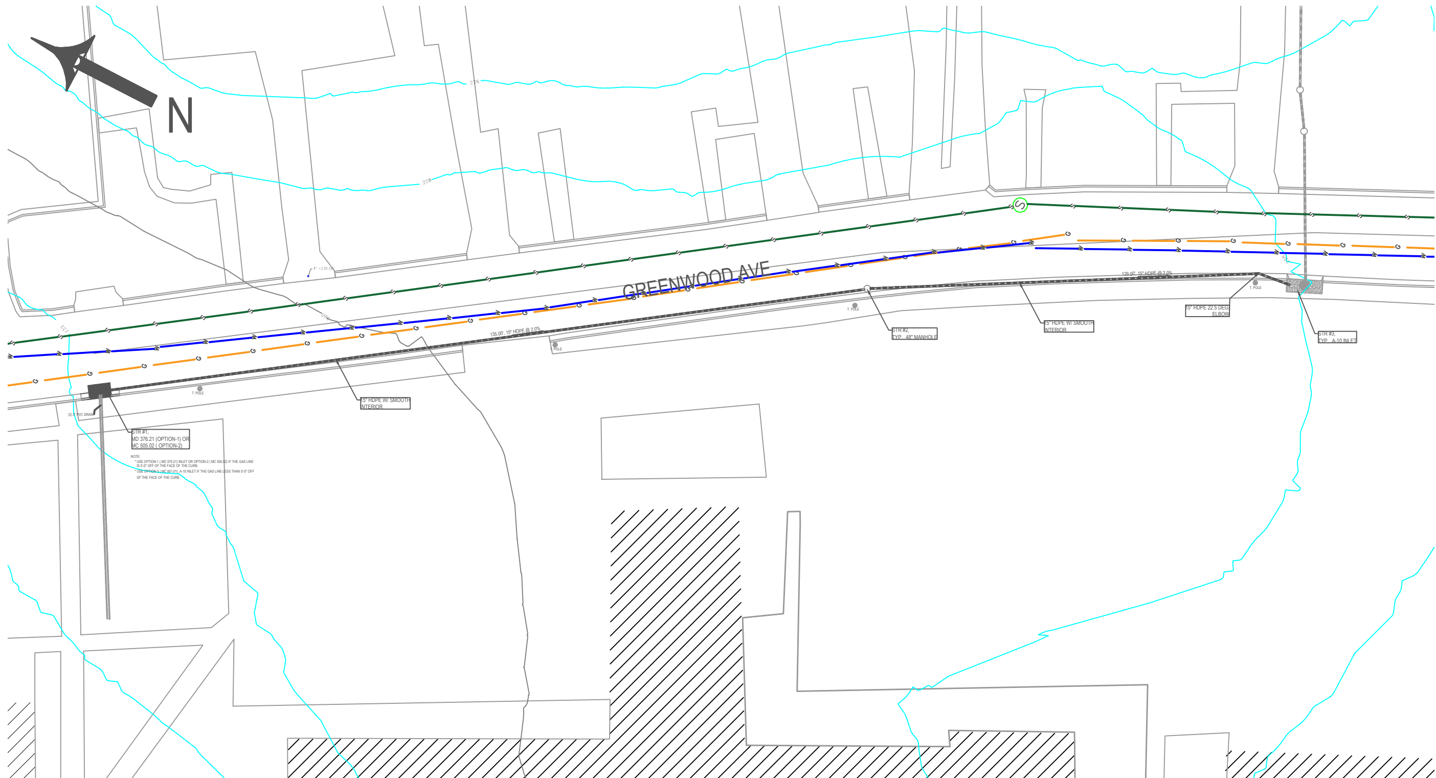
1 SW-4 STORM DRAIN SYSTEM (STR-1 THRU STR-3) PLAN SCALE: 1" = 30'-0"
