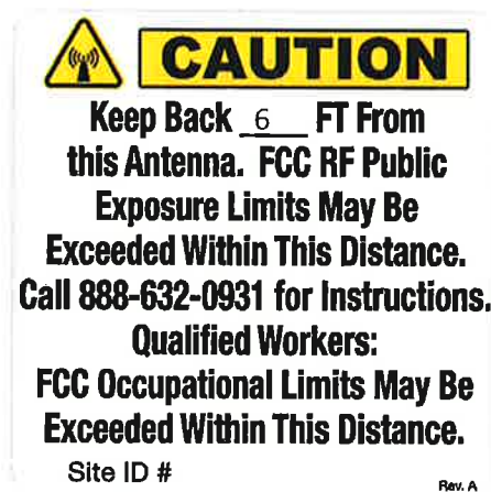
Figure 4. Recommended RF Alert Signage
